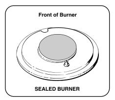
Your new cooktop features four or five sealed gas burners. On Models GGS30/36/365, GGSCV30/36/365, SGS30/30G and SGSCV36G you have two 9,100 BTU/HR burners, two 11,000 BTU/HR burners and on the GGSCV365 or GGS365 there is one 6,500 BTU/HR burner. On Models GGN30/36/365 and SGN30/36 there are two 11,000 BTU/HR and two or three 6,500 BTU/HR burners. Each burner is sealed to the cooktop for easier cleaning.
